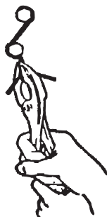
Stretch wires and twist approx. 4 times
