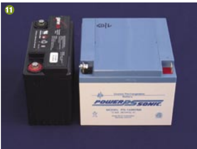
Weighing only 10.6 pounds, this compact 13-amp-hour Genesis battery is sealed and capable of easily starting a Rotax 912ULS. The blue-topped Power-Sonic battery weighs 16 pounds and is twice the size, but at 26 amps has double the capacity. Both batteries do a great job of cranking the high-compression 912ULS engine.
