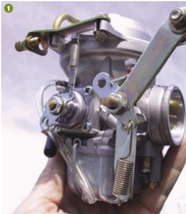
The Bing 64 constant velocity carburetors are sprung to full throttle on the 9-series engines. This carb was photographed at full throttle. The vent line must be vented to the same pressure air as that entering the carburetor.
