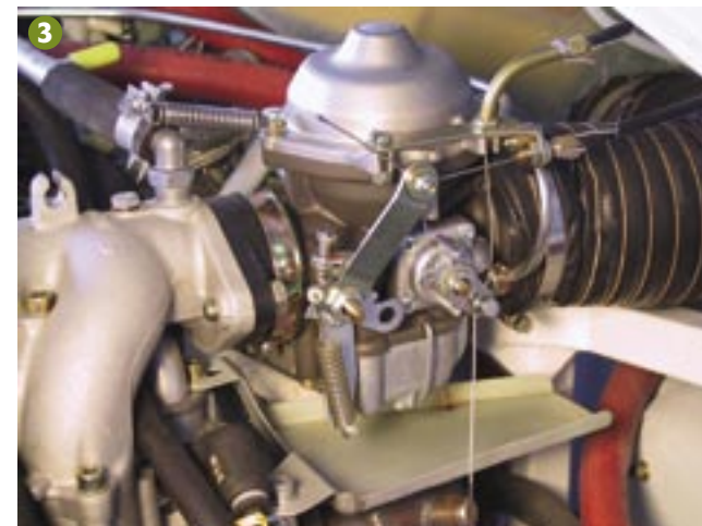
Some airframe manufacturers provide their own under carb drip tray/heat shield as does Flight Design on its CT.
