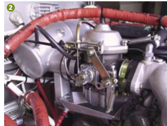
When using the Rotax air box, or any air box, the carburetor vent lines must be connected to the air box so the pressure in the float chamber will be the same as that of the air entering the carburetors. Note the Rotax under carb drip pan/heat shield that comes with the Rotax air box assembly.
