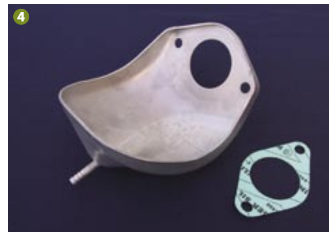
This under carb drip tray/heat shield comes standard as part of the Rotax 914 engine package, Rotax Part No. 874 300. It can be purchased separately for installation on the 912UL and 912ULS.
