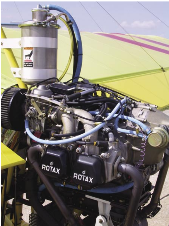
The oil tank on this 912UL engine installation is mounted higher than ideal. On some pusher installations, it can be difficult to locate the oil tank at the recommended height.
