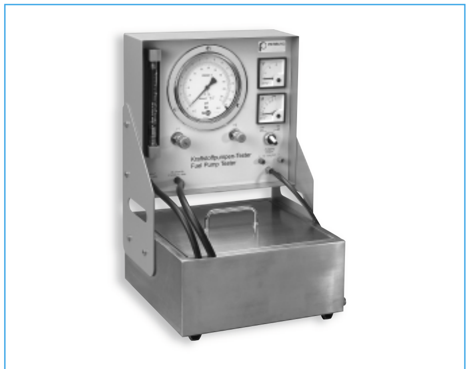
Figure 39 Fuel pump tester 4.07360.60.0
