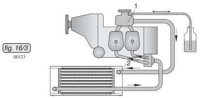
The sensor may be installed in a "TEE" inline with the fluid hose or the expansion tank may be modified to attach the sensor (not supplied by BRP-Rotax).
