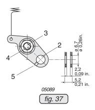
connection for starting carb (choke) actuation (2)
