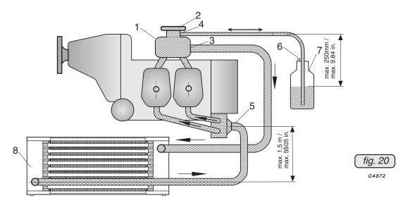
For proper operation of the cooling system the expansion tank (1) with pressure cap (2) has to remain for all possible engine positions on the highest point of the cooling circuit.
