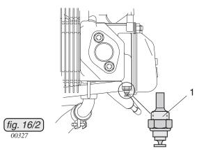
The measuring of the coolant exit temperature is performed using a seperate sensor, which has to be installed in the line between expansion tank (1) and radiator inlet (2).
