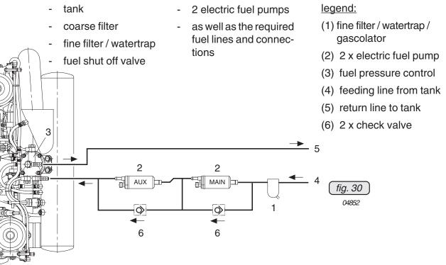
Only the following connections per fig. 30 have to be established:
