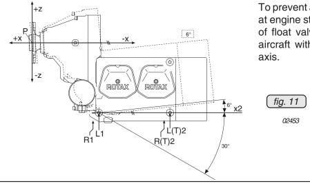
To prevent a possible hydraulic shock at engine start, ensure proper closing of float valves. If in doubt, park the aircraft with inclining propeller shaft axis.
