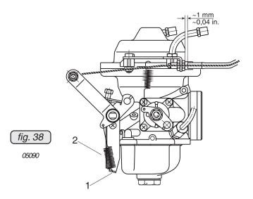
▲ WARNING: With throttle lever not connected the carb will remain fully open. The home position of the CD-carburetor is full throttle!
