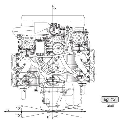
**Tolerated roll deviation of Yaw tolerance:**  $\pm 10^{\circ}$  (see fig. 13)
