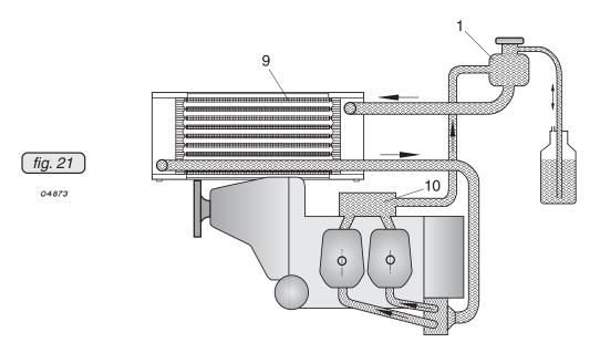
In an installation as depicted with the radiator (9) in a higher position than the standard supplied expansion tank, a water accumulator (10) has to fitted instead of the expansion tank. Additionally a suitable expansion tank (1) has to be installed at the highest point of the cooling circuit.
