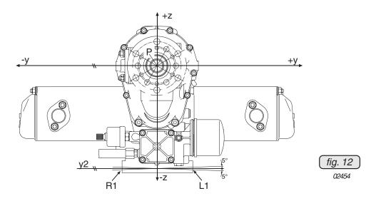
Tolerated roll deviation of parallelism: .....  $\pm 5^{\circ}$ . (see fig. 12)
