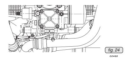
Oil pump inlet nipple (1.1): outside dia ...... 13,2 mm (0.52 in.) slip-on length ..... max. 21 mm (0.83 in.)
